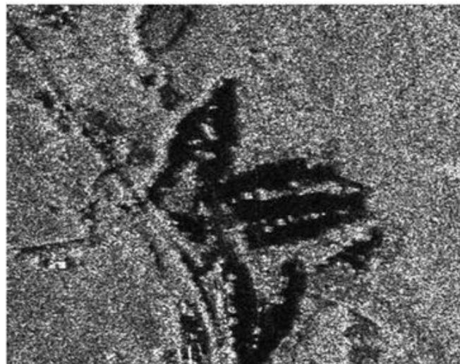
Speckle noise in satellite radar image
