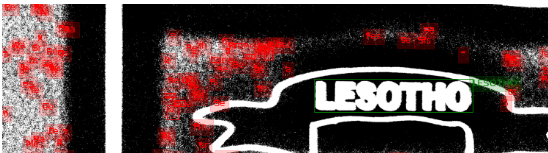
Figure 3.2: Tesseract mistakes background texture for text. Red rectangles and characters denotes predicted words. Part of an preprocessed image from CTW1500 dataset.
